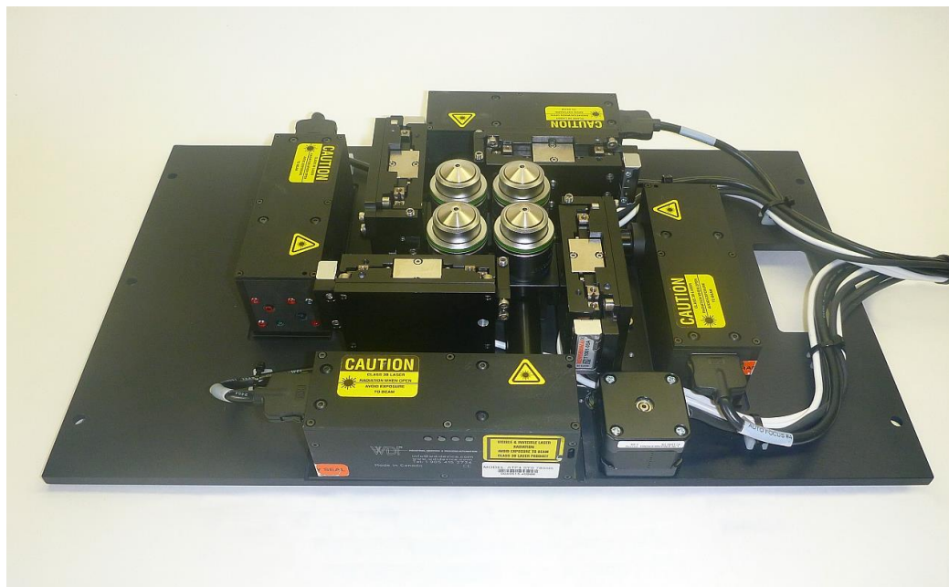
Fig.1 Quad array of 20X, 0.8 NA autofocusing objectives
