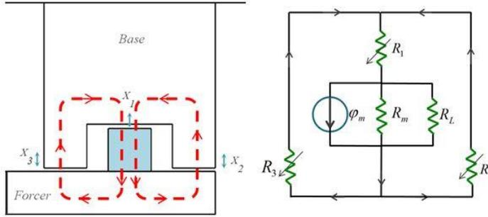
Fig. 3. System top view including magnetic path shown in dotted lines .
