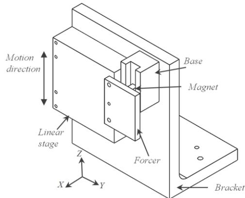
Fig. 1. Basic passive magnetic counterbalance configuration.
