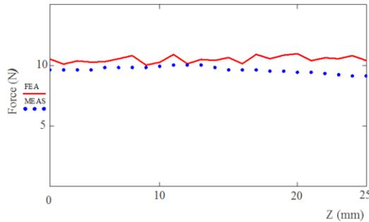
Fig. 4. The net force in Z direction. The solid line is the FEA results and the points are measured data.
