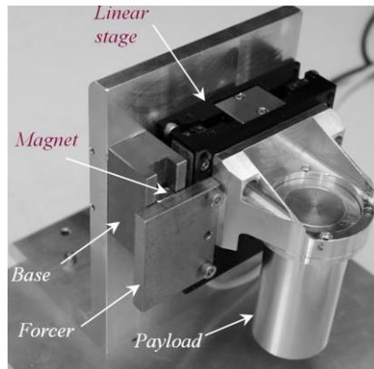
Fig. 2. Experimental prototype.
