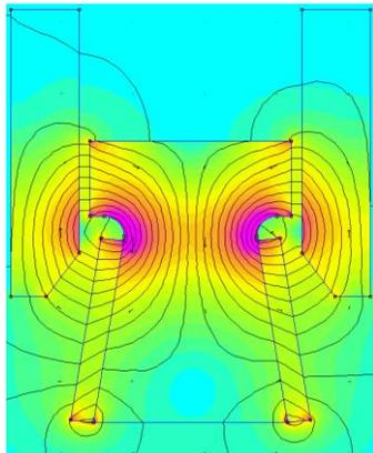
Fig. 5. FEA simulation for alternative design without normal force.
